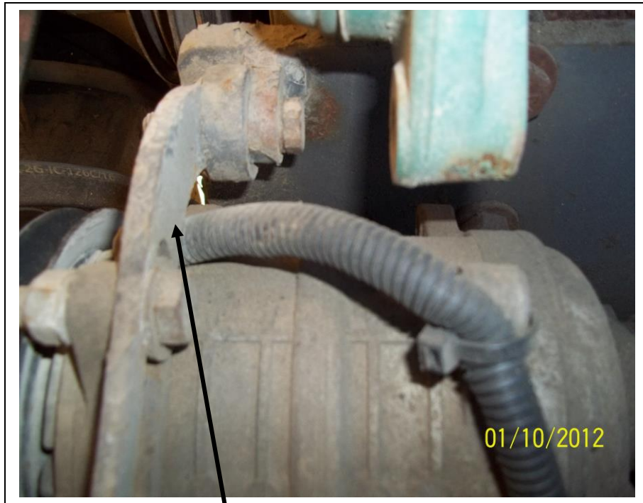
This tightener bracket supplied in kit
