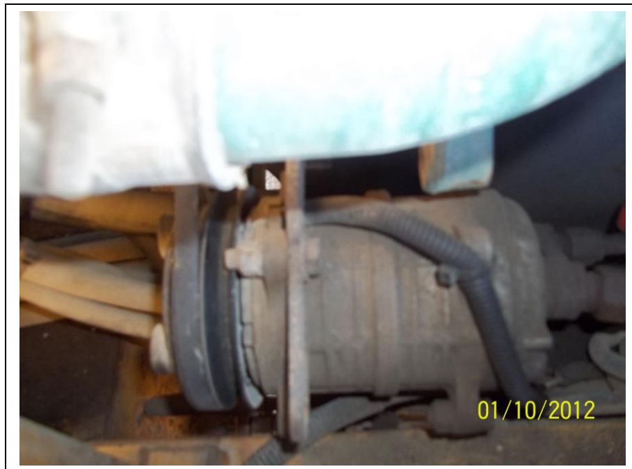
The mounting tabs for the compressor should already exist on the large engine mount bracket.
