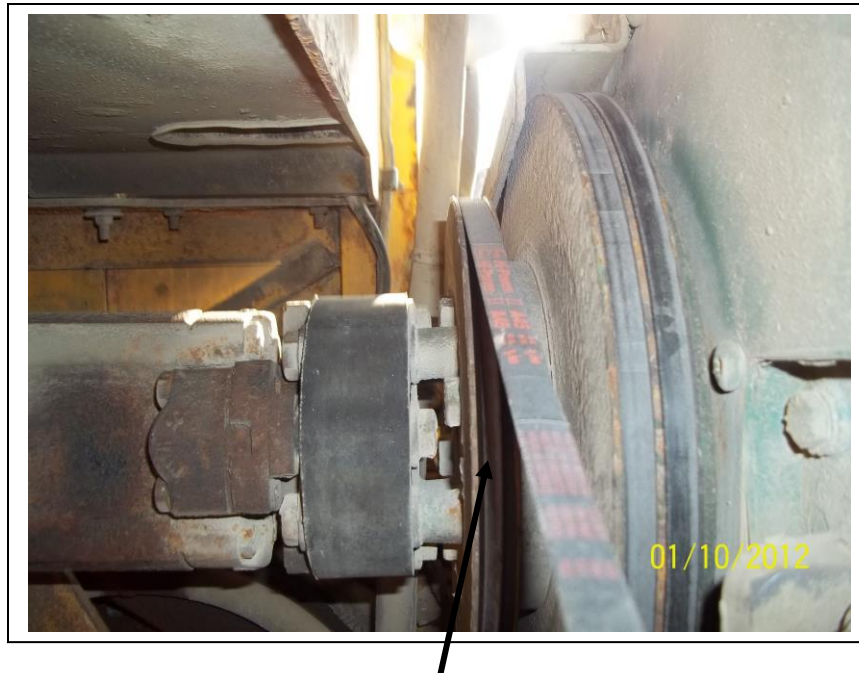
This add on pulley should exist. If not then it will need to be purchased from the dealer.
